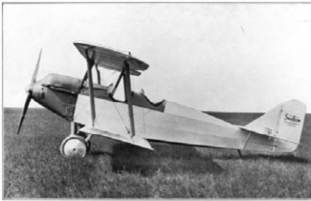
SIDE VIEW OF "NEW SWALLOW" SHOWING HOW PERFECTLY THE SWALLOW IS STREAMLINED. NOTICE THE MOTOR IS COMPLETELY COWLED MAKING MINIMUM FRONTAL RESISTANCE
