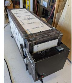
In the best homebuilder traditions of EAA, this presentation will cover the underlying motivation for - and the construction, debugging, and troubleshooting of - a homebuilt oven for solution heat treatment of aluminum.
