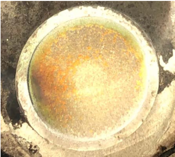
Hot spot (greenish in color) at 8 o'clock on the #3 exhaust valve face.
