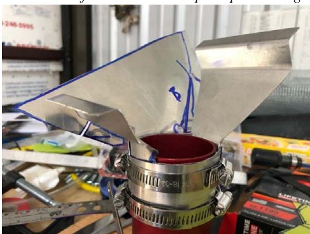
Fabricating a transition duct for the carburetor
