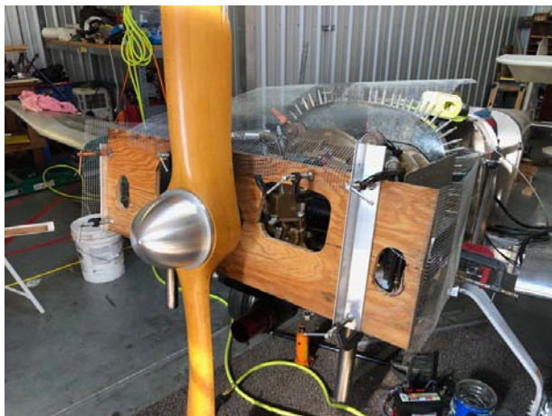
Wooden form that will help shape cowling
