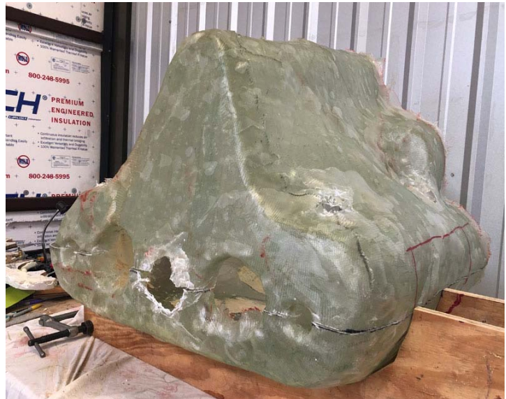
Upper piece of original cowl getting the inside smoothing treatment with epoxy and microballoons to make it a good shape and surface as a mold for the fiberglass cloth layers of the next version of the cowl.
