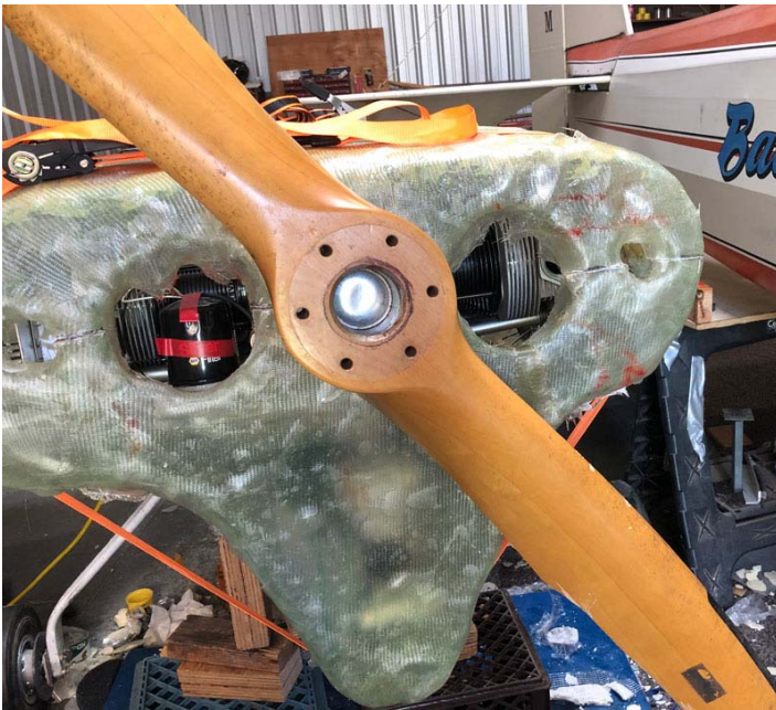
Cowl version 1 as constructed by laying up fiberglass cloth on a foam plug cut to surround the engine.
