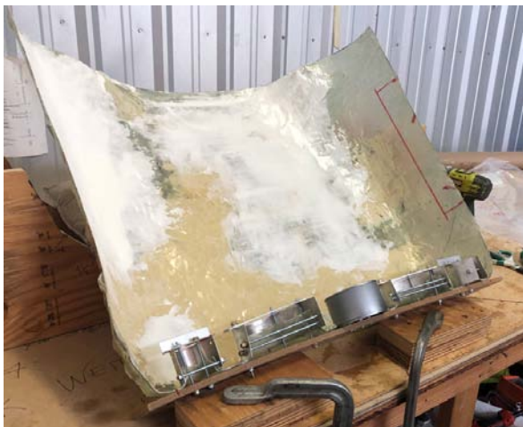
Upper piece of original cowl getting the inside smoothing treatment with epoxy and microballoons to make it a good shape and surface as a mold for the fiberglass cloth layers of the next version of the cowl.
