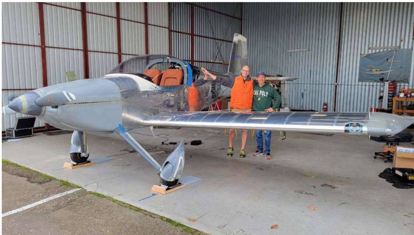
Greg Hansen and Matt Brenner with the RV-14 on its tiptoes for weighing.
