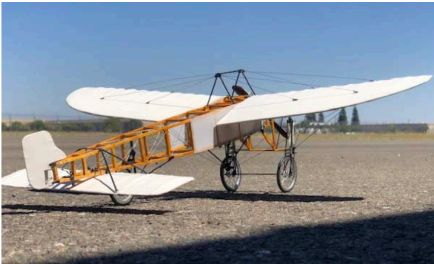
Bleriot XI. 1909, Anzani 3-Cylinder Engine, 25 HP.
